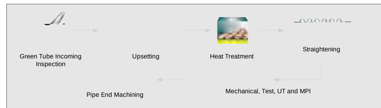
Drill Pipe Welding Flow Chart
